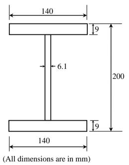
The plastic section modulus about the weaker axis (in cm<sup>3</sup>, up to one decimal place) is
