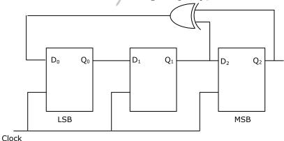
Which one of the following is the correct state sequence of the circuit? (a) 1,3,4,6,7,5,2 (b) 1,2,5,3,7,6,4 (c) 1,2,7,3,5,6,4 (d) 1,6,5,7,2,3,4
