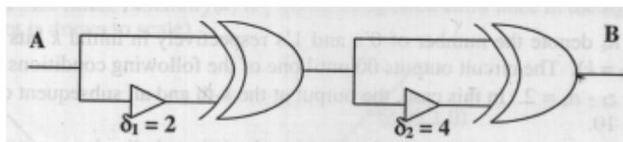
The non-inverting buffers have delays  $\delta_1 = 2$  ns and  $\delta_2 = 4$  ns as shown in the figure. Both XOR gates and all wires have zero delay. Assume that all gate inputs, outputs and wires are stable at logic level 0 at time 0. If the following waveform is applied at input A, how many transition(s) (change of logic levels) occur(s) at B during the interval from 0 to 10 ns?
