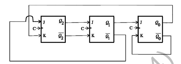
The above synchronous sequential circuit built using JK flip-flops is initialized with  $Q_2Q_1Q_0 = 000$ . The state sequence for this circuit for the next 3 clock cycles is
