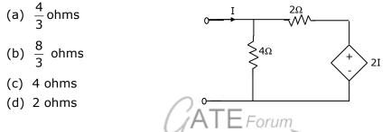
2.3. The impedance seen by the source in the circuit in Fig.2.3, is given by
