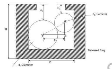
The distance  $H_2$ =35.55 mm and  $H_1$ =20.55 mm. The diameter (D, in mm) of the ring gauge is \_\_\_\_\_
