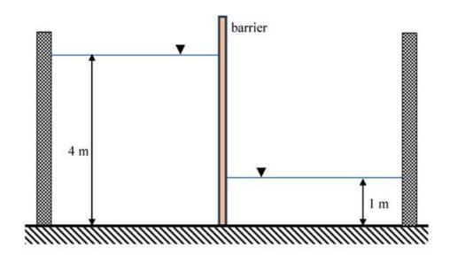
Taking the density of water as 1000 kg/m³, and the acceleration due to gravity as 10 m/s², the maximum absolute bending moment developed in the cantilever is \_\_\_\_\_ kN·m (round off to the nearest integer).
