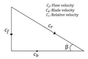
The diameter at this section is 3 m. The hub and tip diameters of the blade are 2 m and 4 m, respectively. The water volume flow rate is  $100 \text{ m}^3/\text{s}$ . The rotational speed of the turbine is 300 rpm. The blade outlet angle  $\beta$  is \_\_\_\_\_ degrees (round off to one decimal place).
