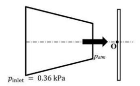
The inlet and outlet areas of the nozzle are 0.1 m<sup>2</sup> and 0.02 m<sup>2</sup>, respectively. Take air density as constant and equal to 1.2 kg/m<sup>3</sup>. If the inlet gauge pressure of air is 0.36 kPa, the gauge pressure at point **O** on the plate is \_\_\_\_\_ kPa (round off to two decimal places).
