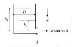
Q. 21 Water discharges steadily from a large reservoir through a long pipeline, as shown in the figure. The Darcy friction factor in the pipe is 0.02. The pipe diameter is 20 cm and the discharge of water is 360 m<sup>3</sup>/h. Water level in the reservoir is 10 m and acceleration due to gravity  $g = 10 \text{ m/s}^2$ . If minor losses are negligible, the length L (in meters, up to one decimal place) of the pipeline is
